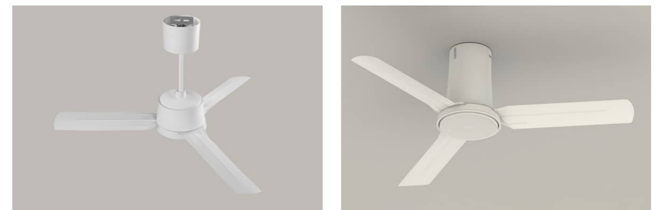
Figure 11. Vortice Nordik eco ceiling fan before (left) and after (right) the redesign. Without jeopardizing the fans' performances (i.e. air flow generated), the blade-to-ceiling height was reduced to 30cm to enable the installation of the ceiling fans also in rooms with internal height down to 260cm, which is a common situation in recent and brand-new residential buildings in Europe.
